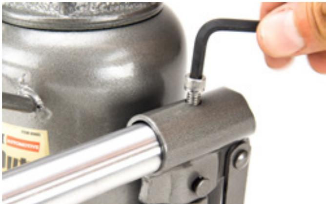
Tighten the Pump Handle in place.
