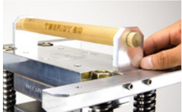
Use remaining long Allen Screws to tighten the second bracket in place.
