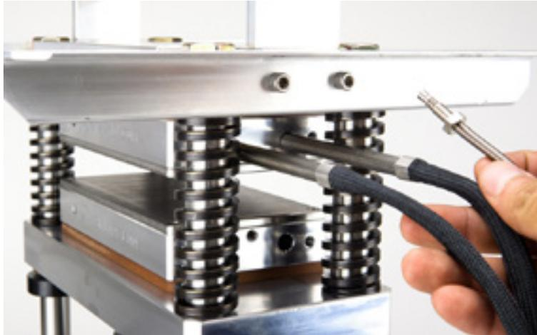
There is a thermocoupler that tags along with each set of heaters. These help in giving an accurate temperature reading back to the controller. The need to be threaded into the middle hole on each plate.
