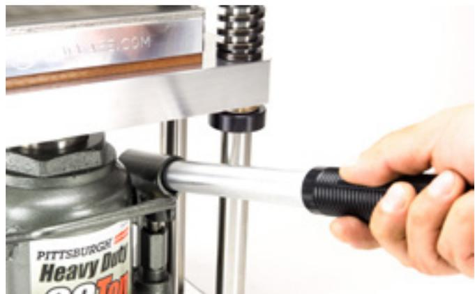
Align hole in handle with the pump insert hole
