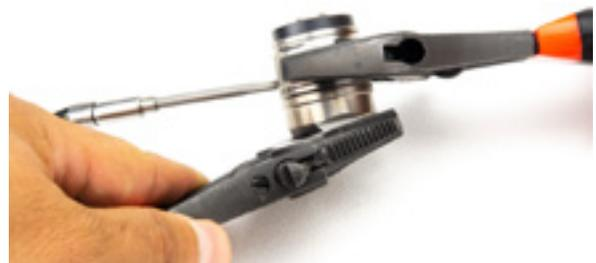
The wrenches should provide enough force to unscrew both parts from each other.
